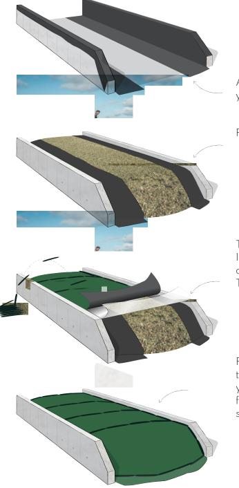
Apply **Triowall** film to protect your silo walls
